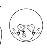
This is available as a rear mounted factory fitted option. The unit contains a 6mm Dia. "festoon" style lamp available in 6V, 12V or 24V.
