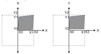
X0 = Start value of input X1 = Elbow value of input X2 = End value of input Y0 = Start value of output Y1 = Elbow value of output Y2 = End value of output
