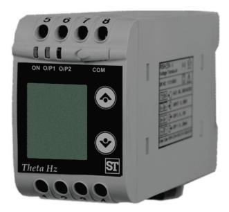
Theta Hz the transducer is used for frequency measurement. The output signal is proportional to measured frequency and is either load independent DC Current or load independent DC Voltage..
