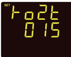
Fig 3-36 RO2 Alarm Delay Setting
