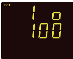
Fig 3-3 Full range shunt setting
