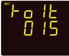
Fig 3-30 RO1 Alarm Delay Setting
